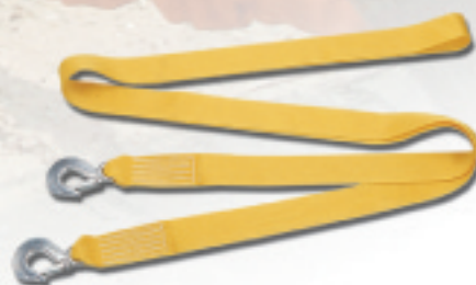
Item No. SP-30 Width : 2" Extension length: 4 ~ 8 M Breaking strength (B/S): 3000 KGF Material : Polyester
