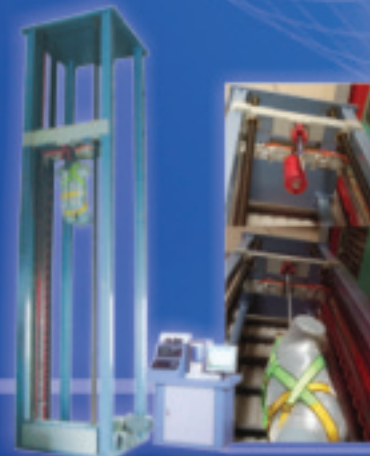
Safety belt impact testing machine, high 6 meter
