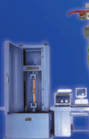
20t computer type universal testing machine
