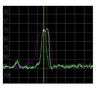
A view trace and reference trace can be displayed in addition to the live trace using contrasting colours for clarity. Any number of traces can be saved to memory and rapidly recalled to the screen. Trace states are saved in addition to the traces and can be recalled separately.
