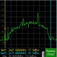
The markers can be set to specified frequency values, scrolled across the screen, or set to automatically find peaks. A peak tracking mode is also provided which will track the highest peak in the sweep despite changing frequency. Marker amplitude readout can be in graticule units (dBm or dBµV) or in linear units (mV or µW).
