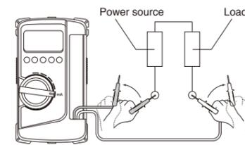
In making measurements, connect your DMM in series with an object to be measured. Do not apply signals exceeding the maximum rated input current.
