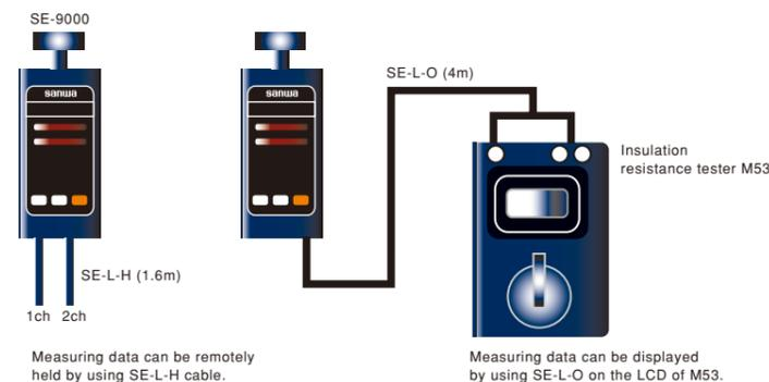
Measuring data can be remotely held by using SE-L-H cable.
