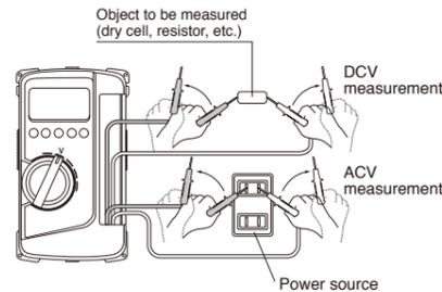
In making measurements, connect your DMM in parallel with an object to be measured. Do not apply signals exceeding the maximum rated input voltage.
