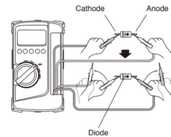
When the black test lead is connected to the cathode side of the diode and the red test lead to the anode side, the forward voltage can be measured. In contrast, if the black test lead is connected to the anode side of the diode and the red test lead to the cathode side, the reverse voltage can be measured and "OL" display appears.
