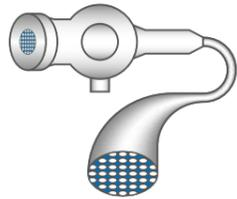
In fiberscopes, also called flexible borescopes, the transmission of images and light takes place via image bundles. Image bundles consist of individual fibers which have the same relative position to each other at the input and output. Each fiber transmits a pixel from the objective to the ocular. The quality of the image depends on the number of pixels and the size of each individual fiber. The image bundle systems ensure the flexibility and movability of the probe.
