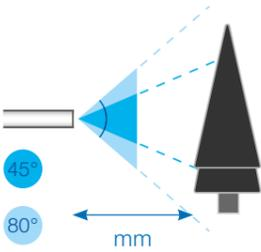
The field of view, also called angle of view or aperture angle, indicates the visible image section. It is specified in degrees. As of 80° and above, it is called a wide angle. The field of view is independent of the direction of view of the borescope/fiberscope. In its standard product range, SCHÖLLY offers fields of view ranging from 30° - 100°.
