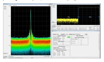
Sophisticated WLAN measurements are easy. On the displayed 802.11g signal, the spectrogram shows the initial pilot sequence followed by the main signal burst. The modulation is automatically detected as 64 QAM for the packet and displayed as a constellation. The data summary indicates an EVM of -33.24 dB RMS, and burst power is measured at 10.35 dBm. SignalVu-PC options are available for 802.11a/b/j/g/p, 802.11n and 802.11ac to 40 MHz bandwidth.
